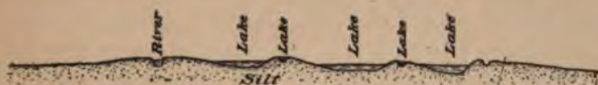
FIG. 454.—Levee lakes developed concentrically in series within meanders of a stream tributary to the Mississippi and flowing upon its delta plain. b and c are examples of the ribbon type of levee lake due to occupation of the abandoned river channel. The larger number of lakes, of which Sip Lake and Texas Lake are examples, have the form of crescents and lie between abandoned levees (from recent map of U. S. G. S.).
